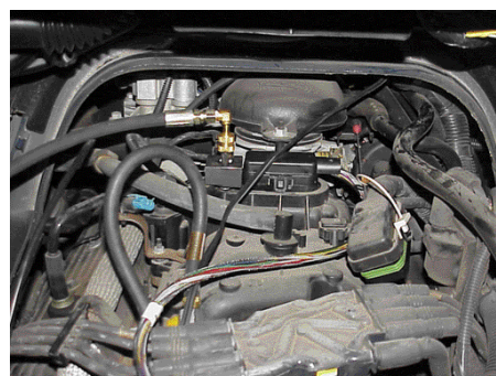
Using recirculation hose -- Jumper block attached to metering body; recirculation hose visible in foreground
