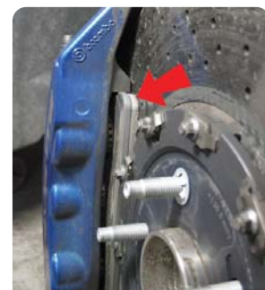
White appearance results from heavier track burnishing
