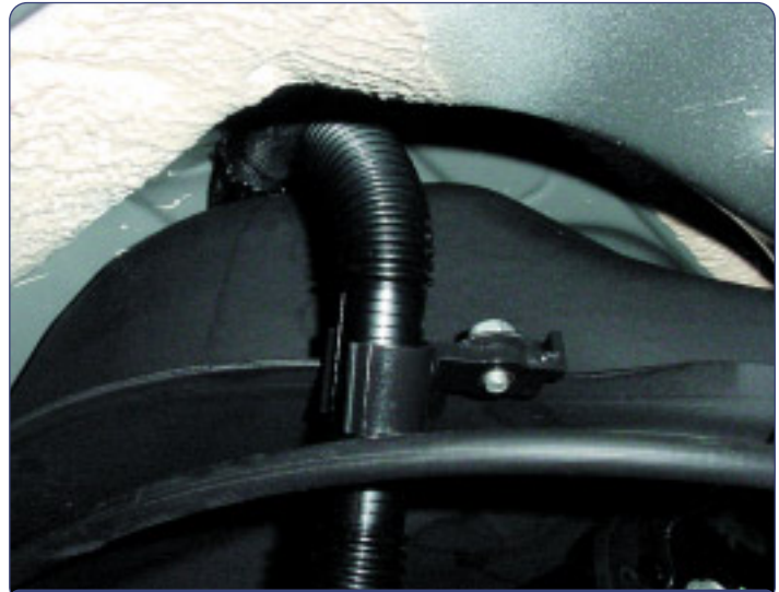
Fuel tank vent hose routing to ORVR valve
