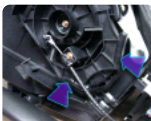
Potential mode cable interference as cam rotates
