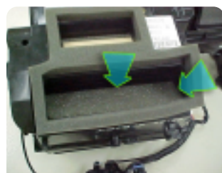
Trim foam that overlaps shape of valve (defrost valve shown)
