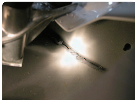
Location of sealant voids
