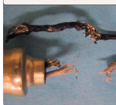
Wire Torn by Use of Improper Socket
