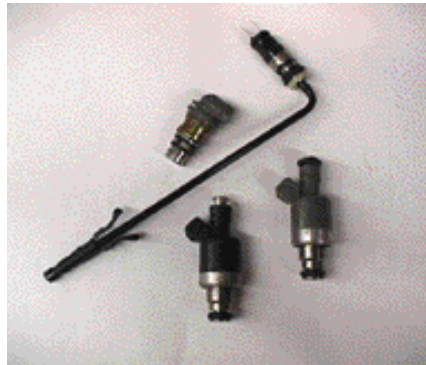
Rochester Multec injectors (MFI, CSMFI) 12-14 Ohms
