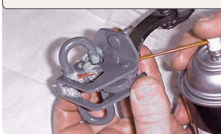
Link removed to show lubrication location
