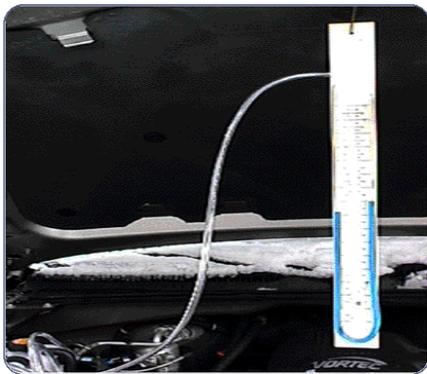
**Homemade Manometer Showing Vacuum at Idle**
