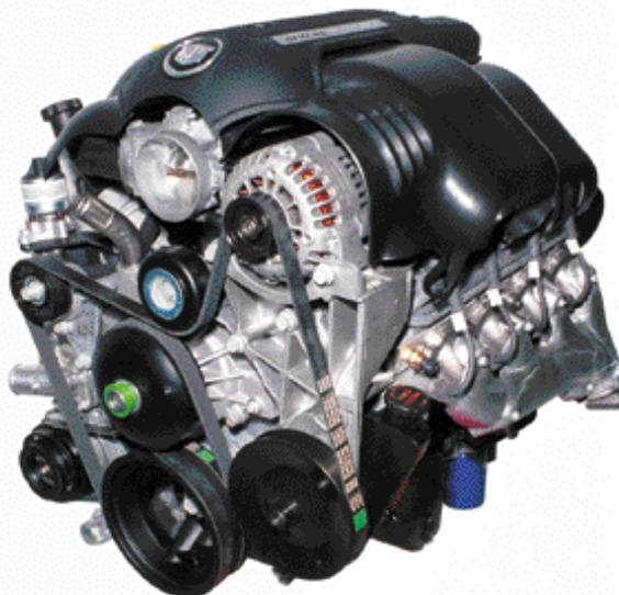
High Output 6000 engine (LQ9). Output is 345 hp, the highest of any SUV in the world. It offers power for passing, hill climbing, and towing.
