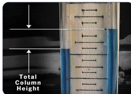
applied to the reference fluid. The total difference in column heights is the reading. Next, observe whether you have pressure or vacuum. Fluid shifting toward the crankcase indicates vacuum, away from the crankcase indicates pressure.
