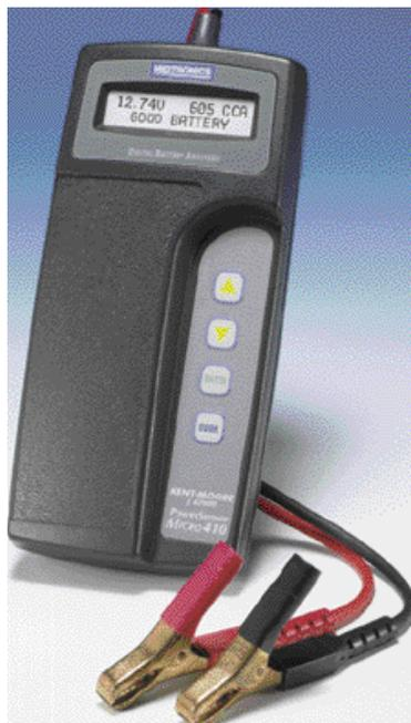
ies that are serviceable and can be charged, without the need to perform a traditional load test. Follow the instructions in the service bulletin.
