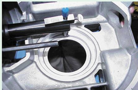
**Picking Up the Location of the Bottom of the Left Side Bearing Bore**
