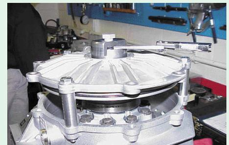
**Measuring Clearance of Right Output Shaft**
