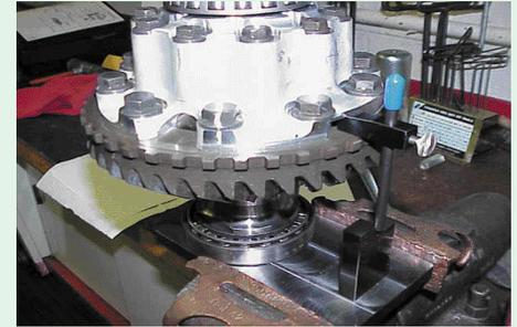
**Measuring Length of Axle Carrier**
