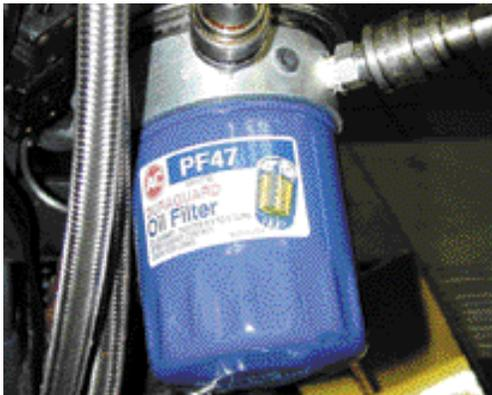
**A conventional oil filter is used, although the braided cooler lines are part of the test setup.**
