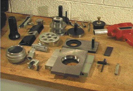
nents of the Getrag-designed rear axle were serviceable only by replacement of the whole unit. Now, a new tool kit from Kent-Moore permits servicing the rear axles in all C5 Corvettes.
