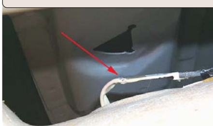
Headliner Removed to Show Wire Location
