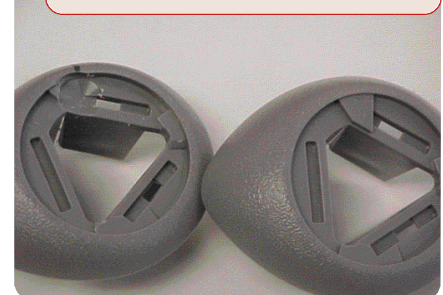
Bezel on left showing drilled out triangular lock
