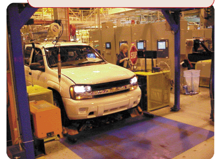
FORI Inspection Station
