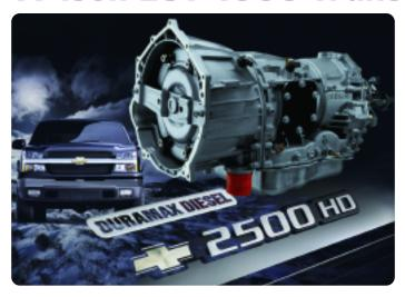
The Allison LCT 1000 automatic transmission is offered in 3/4- and 1-ton Silverado and Sierra trucks with the 8.1L gasoline and 6.6 Duramax diesel engines. This robust transmission offers five forward speeds and one reverse. The forward and reverse gear ratios are accomplished by five clutches.
