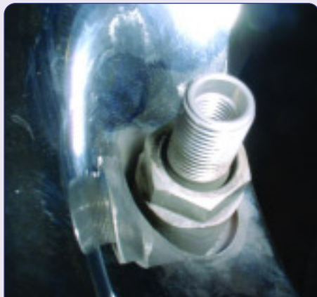
Sensor mounted with valve stem nut
