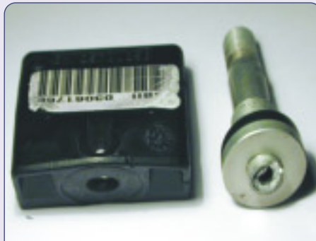
Sensor ruined by tire mounting equipment
