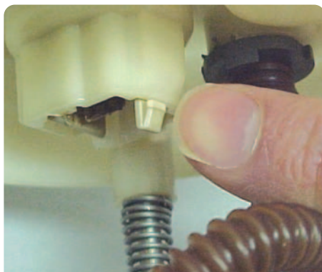
D Depressing lock tab on connector
