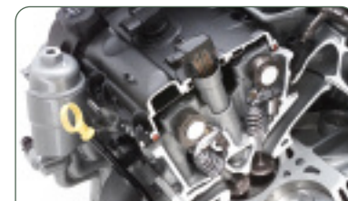
Spark plugs and coils mounted in center of cam cover
