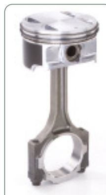
Piston with full-floating wristpin
