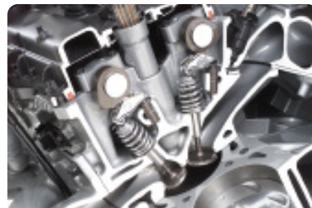
Valve train, showing roller-finger followers and hydraulic lash adjusters
