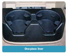
The rear center console cup holders may not retain a cup properly when turning or accelerating. The original liners are cup mats with no retention tabs.
