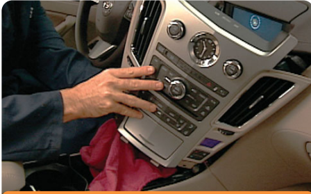
Control Assembly removed
