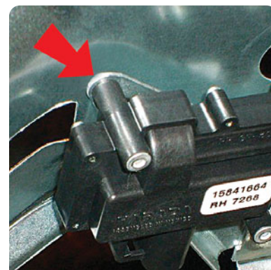
Mushroom end of rivet contacts sliding door inner panel
