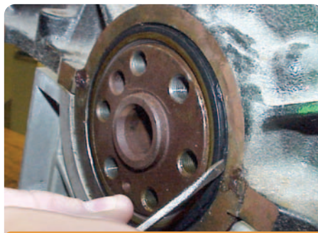
Removing old style seal
