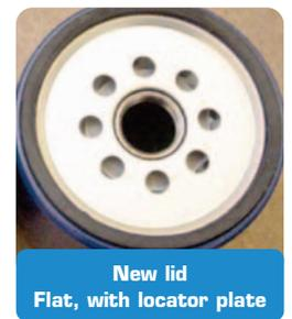
The new locator plate design (flat surface) allows for easier installation in blind applications with no effect to the filter's performance. A rolling change will begin January 27, 2006, with no part number revisions. The first part numbers to be implemented are the 25011520 (PF53) and 19114118 (PF53F).
