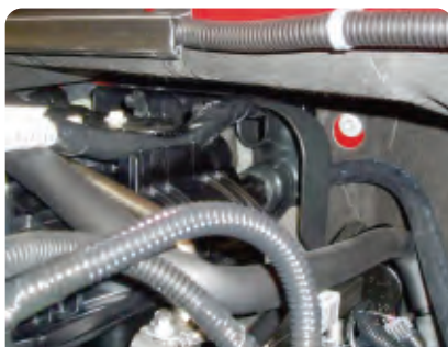
Harness not properly seated in U-channel
