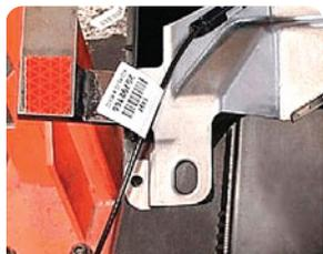
RKE antenna snapped into hole on the passenger knee bolster bracket.
