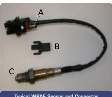
Typical WRAF Sensor and Connector A-Trimming Resistor • B-Resistor Cover C-Sensor
