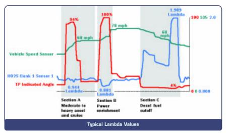
during cruise (Section A). This is because the sensor and the engine controller are in their own closed-loop operation and the lambda value only "drifts" above or below 1.000 as the engine controller makes its fuel trim adjustments. This closed-loop operation between the engine controller and the WRAF sensor is an instantaneous reaction to voltage deviations between the reference voltage circuit and low reference circuit and the resulting oxygen ion exchange via the pumping circuits.
