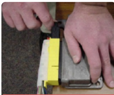
Connector position assurance (CPA)
