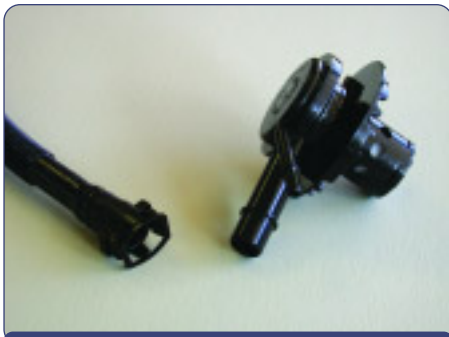
Vapor line between fuel tank and canister
