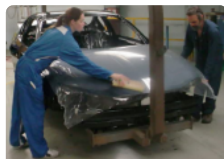
Installation of Transseal at the factory
