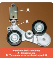
*TIP*: There are two ways to relieve tension on the drive belt, depending on whether the shipping clip is still in place (new tensioner) or the shipping clip has been removed (used tensioner).
