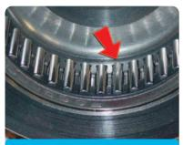
Spalled needle roller
