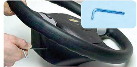
Inserting Allen key
